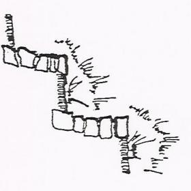
Retaining walls, where necessary, shall be of suitable rock or timer construction and shall not exceed a height of 3 feet without having a step back for planting. This step back will miligate the appearance of the face. These retaining walls shall be planted and maintained to retain an ongoing integrity.
